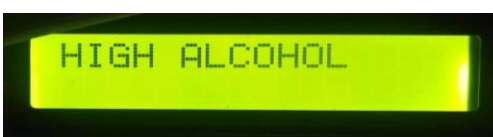
Figure-19. LCD Display when alcohol detected higher than the limit
