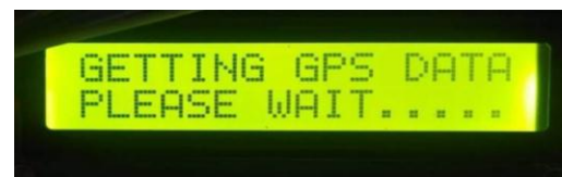
Figure-22. LCD Display when accident detected, and the vehicle is Getting GPS data
