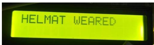
Figure-18. LCD Display when Helmet worn
