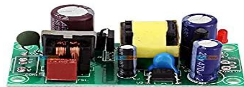
Figure-1. Power supply
