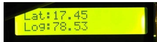
Figure-23. LCD Display when the accident is detected, and the vehicle detects the location
