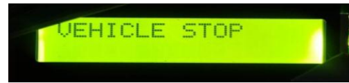
Figure-20. LCD Display when alcohol is detected higher than the limit and then Vehicle is locked
