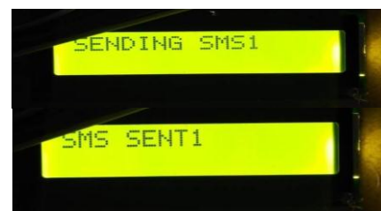
Figure-24. LCD Display when the accident or alcohol is detected, and the vehicle detects the location and that SMS is sent to the required help and family members
