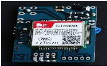
Fig-5: GSM Module
