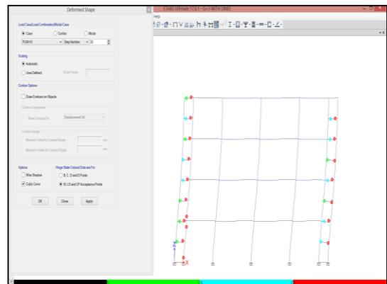
Fig -12: Hinge Formation in 4 Storey RC Building with CFST LCF (4RC\_CFLCF)
