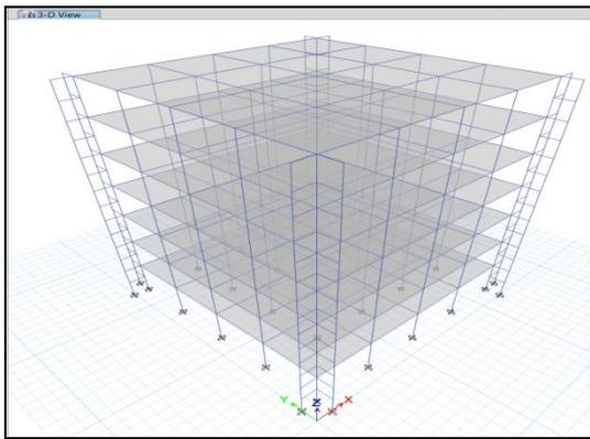
Fig -9: 7 Storey RC Building with CFST LCF (7RC\_CFLCF)
