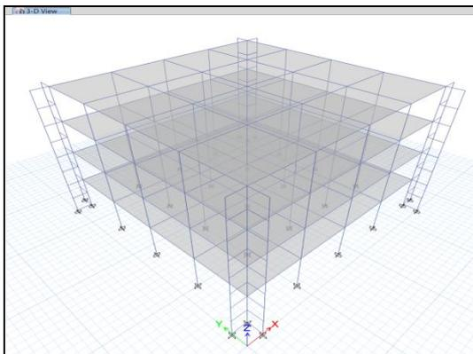
**Fig -4:** 4 Storey RC Building with RC LCF (4RC\_LCF)
