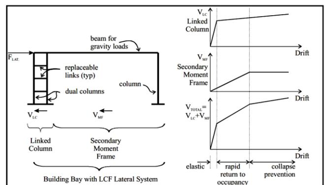
**Fig-1:** Linked Column Frame Elevation and Base Shear Distribution [2]
