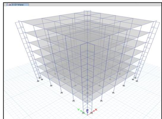
**Fig -8:** 7 Storey RC Building with RC LCF (7RC\_LCF)
