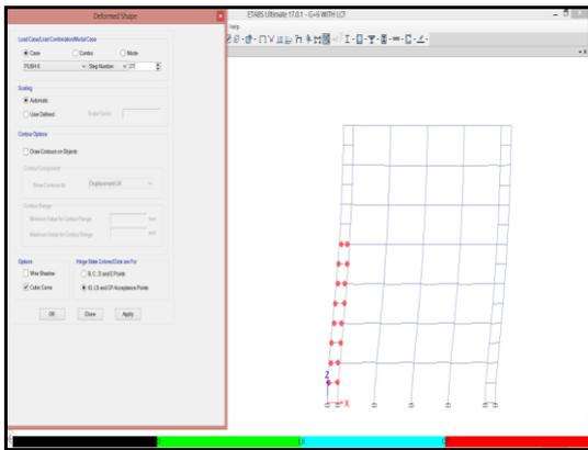
Fig -14: Hinge Formation in 7 Storey RC Building with RC LCF (7RC\_LCF)
