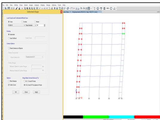
Fig -15: Hinge Formation in 7 Storey RC Building with CFST LCF (7RC\_CFLCF)
