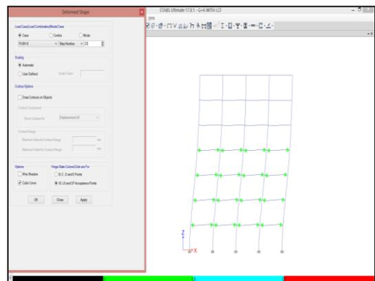
Fig -13: Hinge Formation in 7 Storey RC Normal Building (7RCNB)
