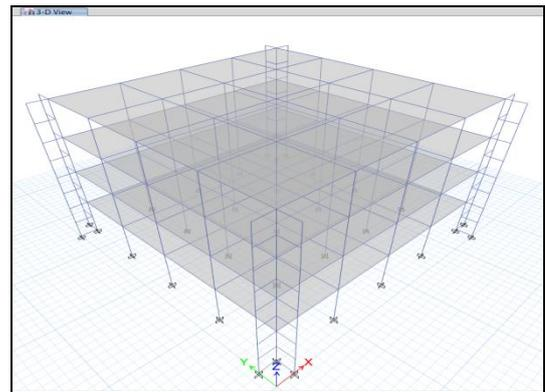
**Fig -6:** 4 Storey RC Building with CFST LCF (4RC\_CFLCF)
