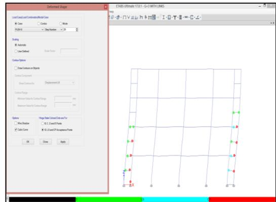
Fig -11: Hinge Formation in 4 Storey RC Building with RC LCF (4RC\_LCF)
