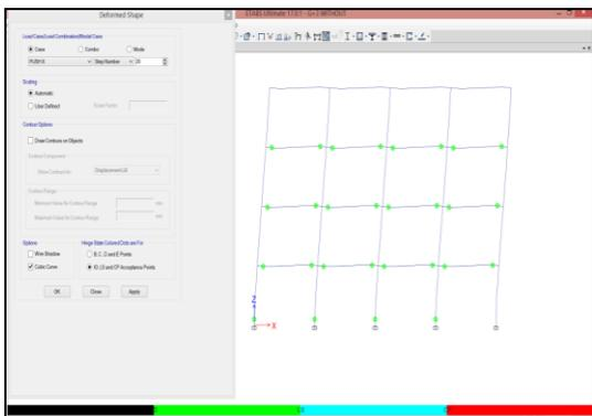
Fig -10: Hinge Formation in 4 Storey RC Normal Building (4RCNB)
