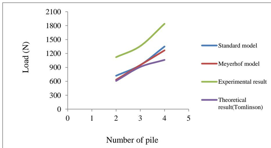
Figure 11 Comparison with theoretical models
