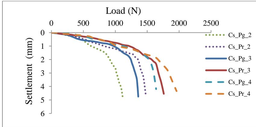
Figure 5 Load vs. Settlement (D3, D4)
