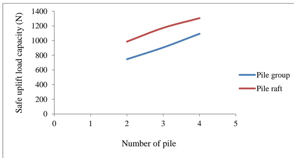
Figure 7 Safe uplift load capacity vs. Number of pile
