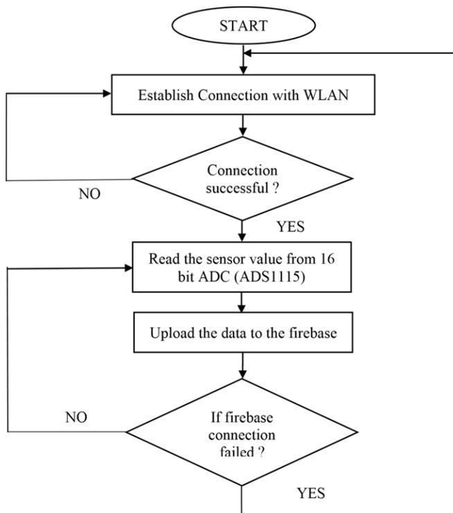
Fig 3.1: flow chart of Arduino program
