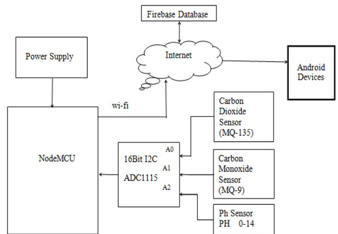
Fig 1.1: Block Diagram of Pollution Monitoring System
