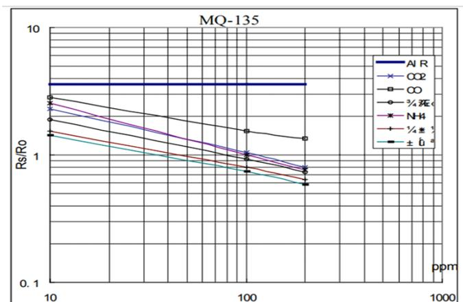
Fig 3.5.1: Logarithmic graph of MQ-135 sensor
