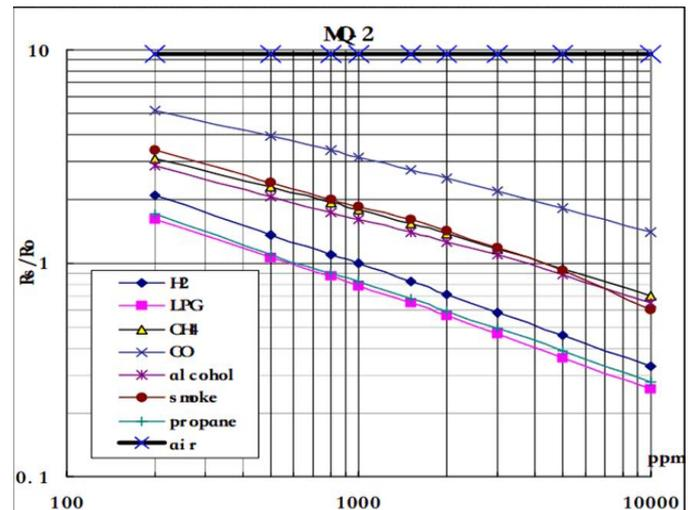
Fig 3.4.1: Logarithmic graph of MQ-2 sensor
