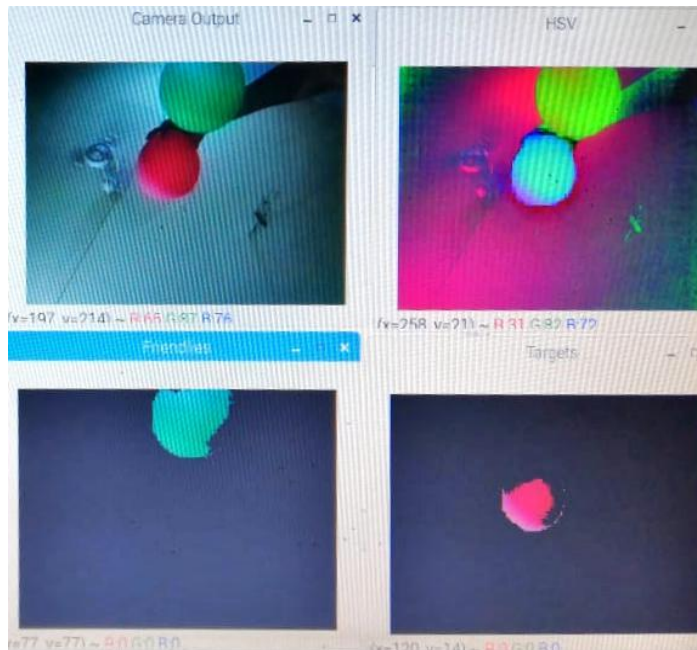
Fig -5: HSV method to detect targets and friendlies
