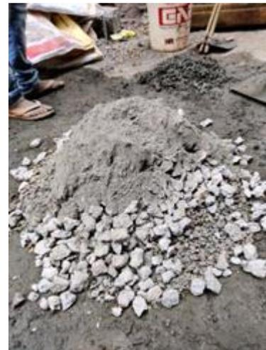
**Fig -5:** Construction & Demolition Waste in Concrete
