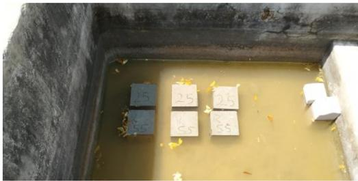
Fig -7: Curing of Cubes
