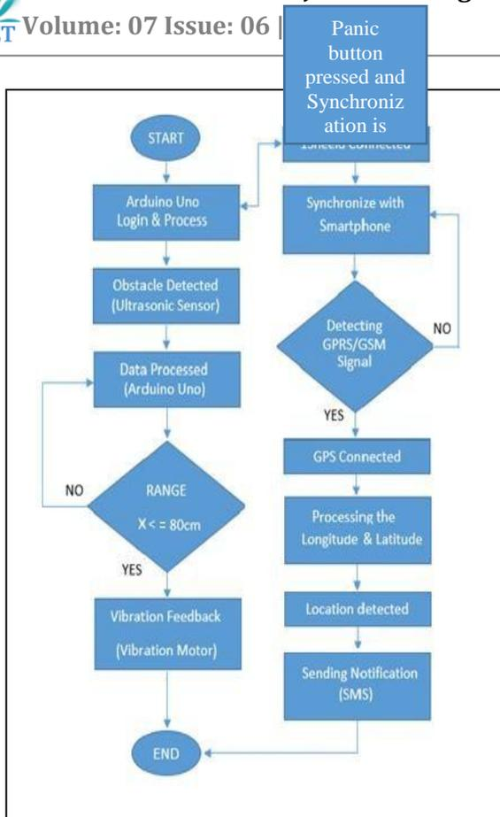
connected to the satellites to fetch the location data, that is, the Latitude and Longitude of the device location. Then this location data is sent to the user family and friends by sending an SMS to the mobile number mentioned in the program code. Thus the person can be tracked and necessary help can be provided.
