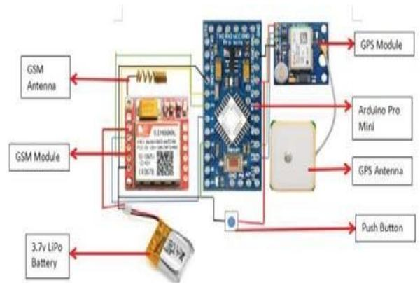
GPS - GSM Circuit Diagram
