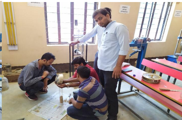
Fig3. Bulking of fine aggregates at lab
