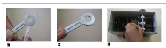
Fig -3: (a) Application of a small drop of bacterial suspension or young fluid culture is at the center of disk. (b) Coating with viscous paraffin oil (c) Application of disk type sample holder in device.
