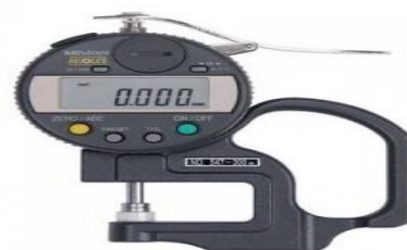
Fig-23. The thickness of rod measuring by mitutoyo 1301 thickness gauge is used quality chuck.
