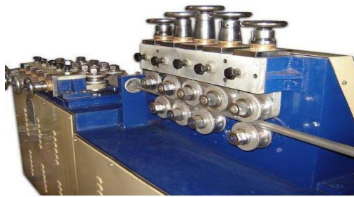
Fig-5: Show the rod straightening process.
