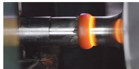
Fig-16: show the welding due to friction.
