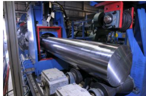
Fig-3: Show the bar peeling process.
