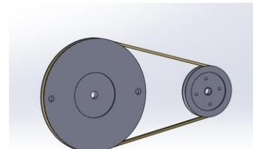
Fig -5: CAD model of Belt-Pulley
