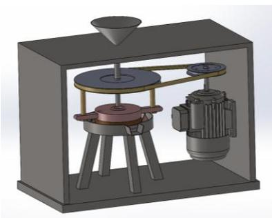
Fig -2: CAD Assembly model of Mechanized quern
