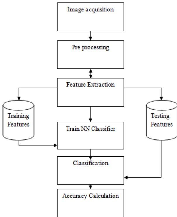
Fig-2: Process Flow Diagram for Proposed Method
