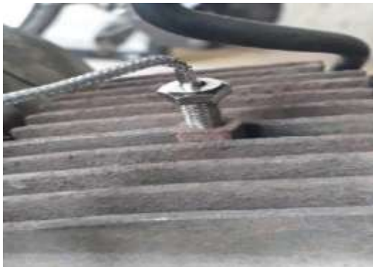
Fig -2: Fixing of Thermocouple
