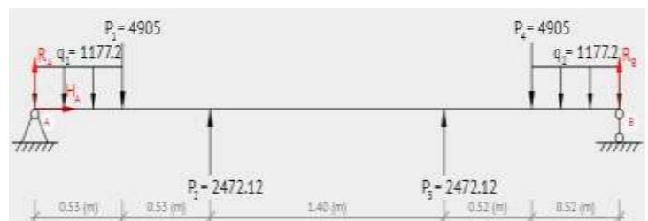
Fig.5.1. Free body diagram
