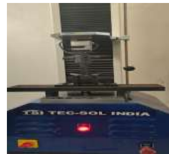
Fig 4.4: Flexural Specimen Loading Position
