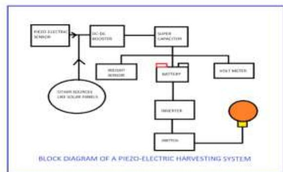
The faces of piezoelectric material, usual quartz, is coated with a thin layer of conducting material such as silver. When stress has applied the ions in the material move towards one of the conducting surface while moving away from the other. This results in the generation of charge. This charge is used for calibration of stress. The polarity of the produced charge depends upon the direction of the applied stress. Stress can be applied in two forms as Compressive stress and Tensile stress.
