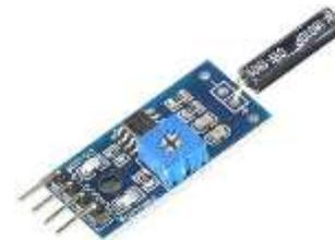
Fig 4.3 Vibration Sensor
