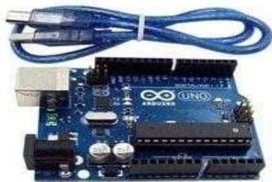
Figure 5: Arduino Uno R3
