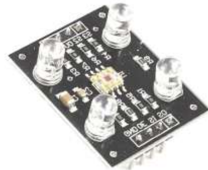
Figure 2: TCS3200 Color Sensor
