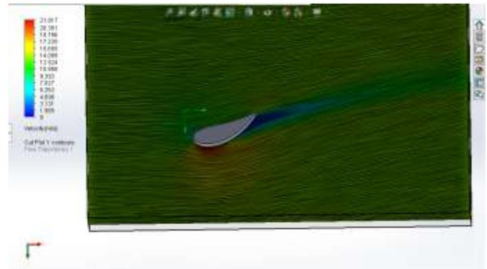
**Figure 5-** Streamline & Velocity Distribution
