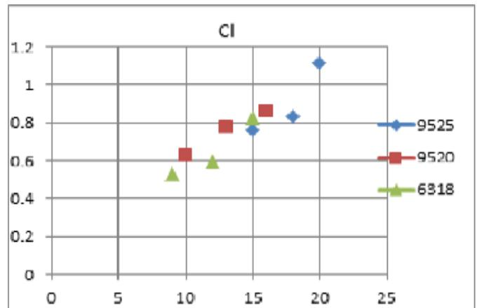
**Chart - 5:**  $C_l$  vs. Alfa for three airfoils
