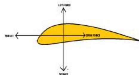
Figure 1- Shape of Airfoil
