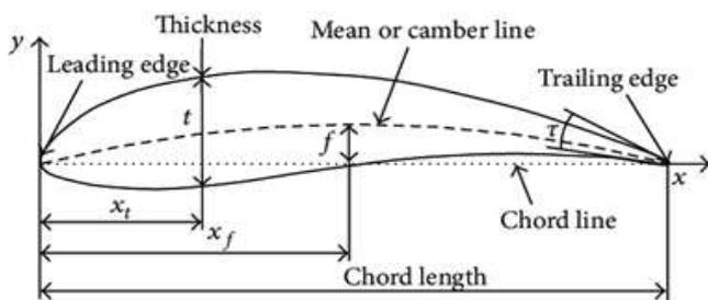
Figure 2- Shape of Airfoil [3]
