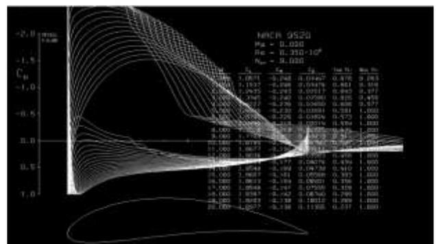
**Figure 3-** Xfoil Graph for NACA 9520
