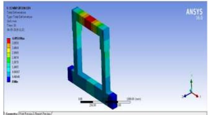
Fig -8: Deformation
