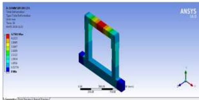
Fig -6: Deformation
