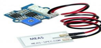
Fig-6: Vibration Sensor Module
