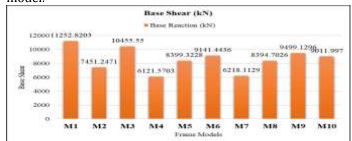
Fig - 6: Comparison of base shear of models
