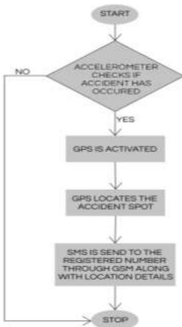
Fig -11: Accident Detection
