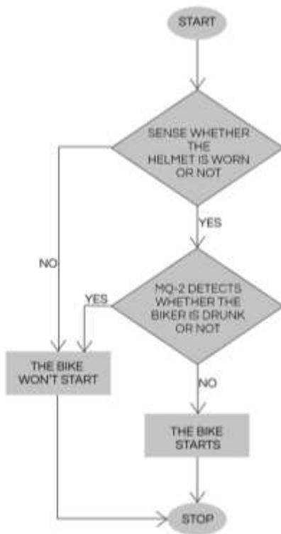
Fig -10: Alcohol Detection
