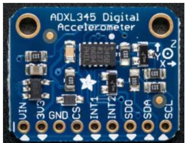
Fig - 4: Accelerometer
