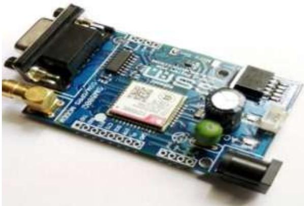
**Fig -8: GSM Module**
