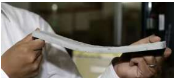
Figure-1: Flexible concrete specimen made by Professor Vector Li
