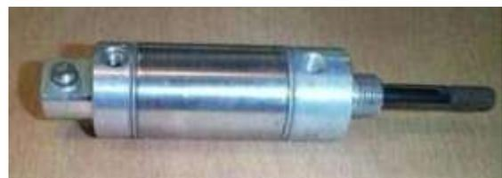
**Fig -2: double-acting cylinder**
