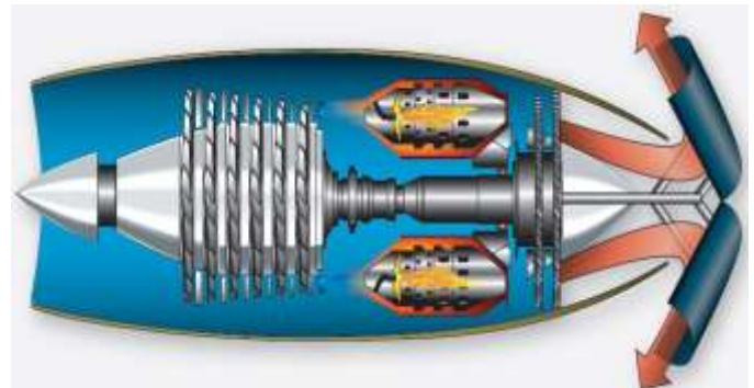
Target type Thrust Reverser
