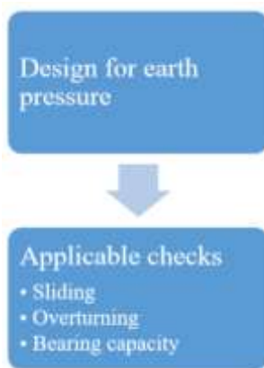
Fig -10: Design steps for Wing wall
