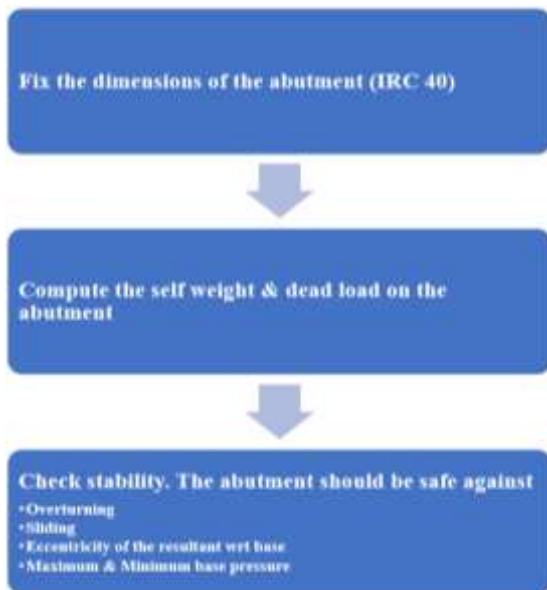
Fig -9: Design steps for Abutment
