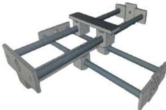
Fig. 3: Design of Cross-Slide
