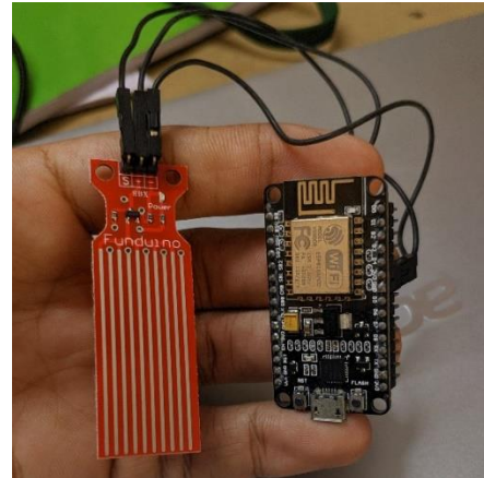
Fig- 5: Water Level Sensor with NODEMCU
