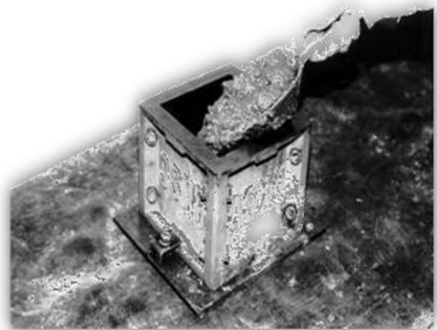
Fig: 8. Placing Of Concrete (a)
