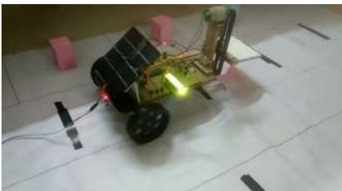
Fig.5: Battery Charging through Solar Panel
