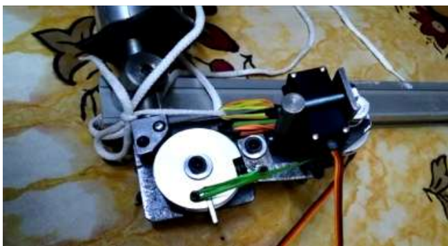
Fig 4.1: 3 Servo motors working together and acting as a Striking mechanism to take a shot
