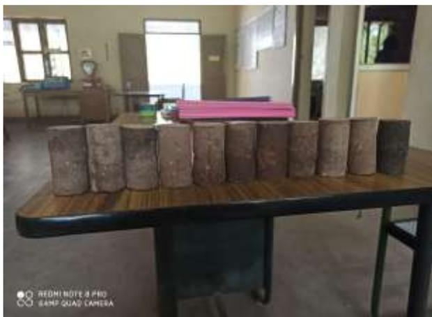
**Fig -3: Unconfined Compressive Strength Test Samples**
