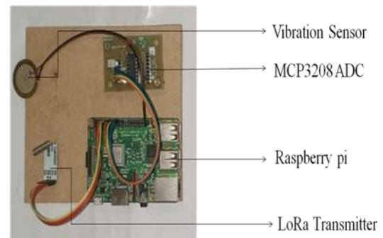
Fig -2: Transmitter Side
