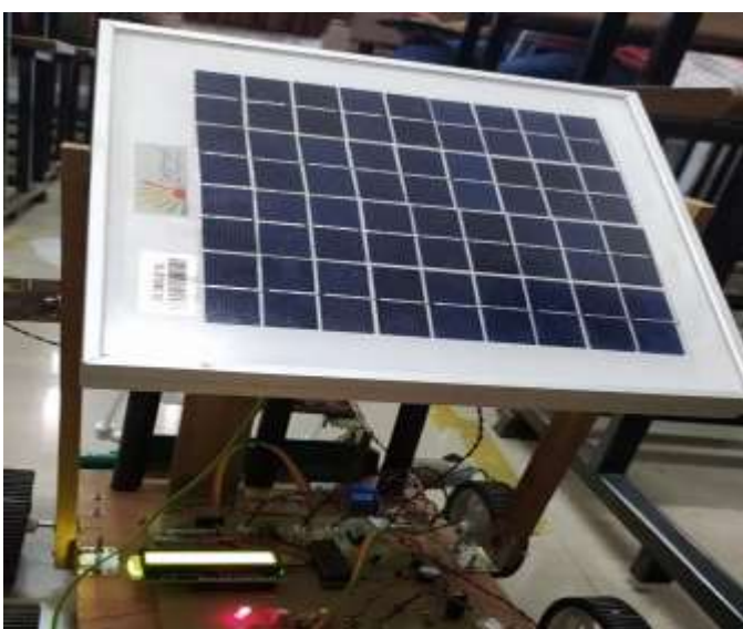
Fig -7: Solar PV Based Charging
