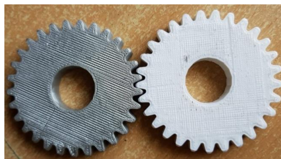
Fig 21: Gears are manufactured by 3D printing
