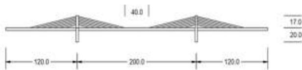
Fig -1: Extradosed bridge with 17 m pylon
