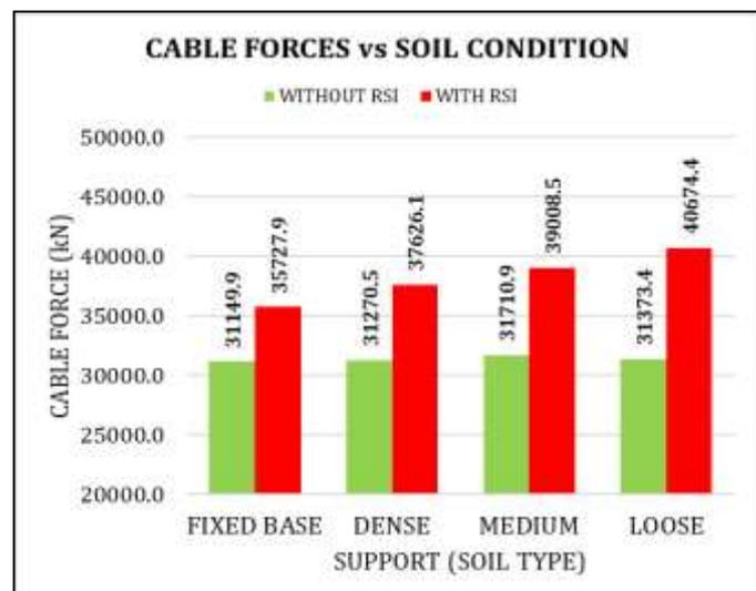
Chart -2: Cable force - 17 m pylon and HSLM A4
