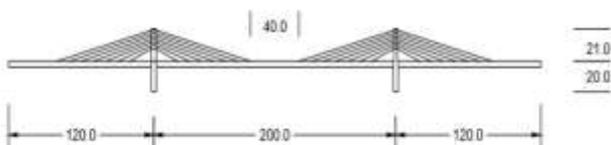
Fig -2: Extradosed bridge with 21 m pylon
