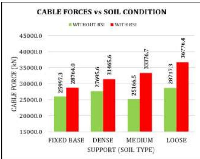
Chart -5: Cable force – 21 m pylon and HSLM A4
