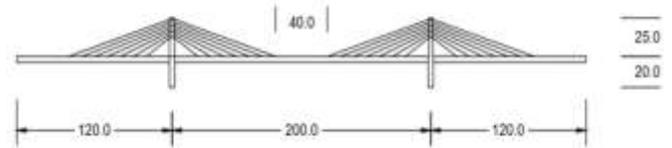
Fig -3: Extradosed bridge with 25 m pylon
