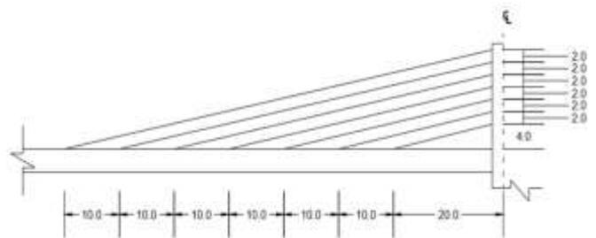
Fig -4: Cable arrangement for 17 m pylon
