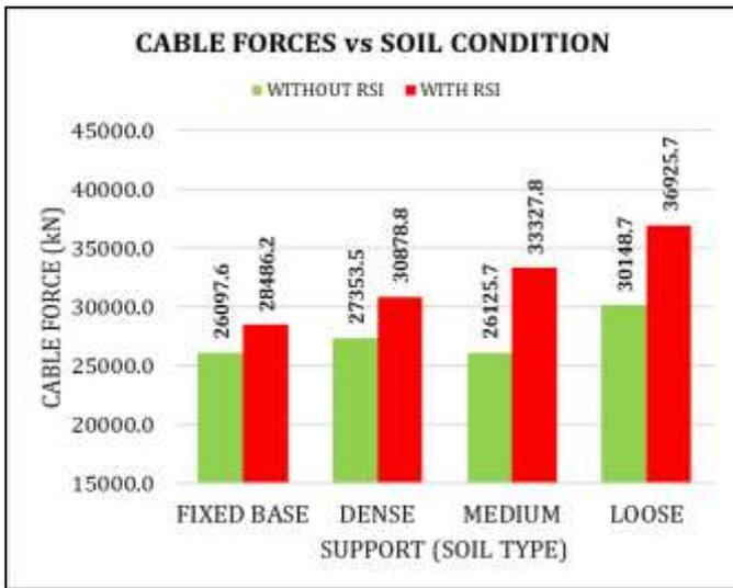
Chart -4: Cable force – 21 m pylon and HSLM A2
