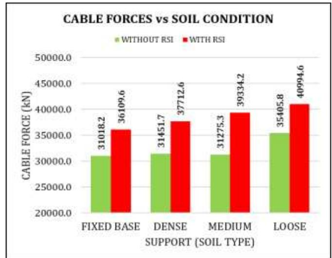
Chart -1: Cable force - 17 m pylon and HSLM A2
