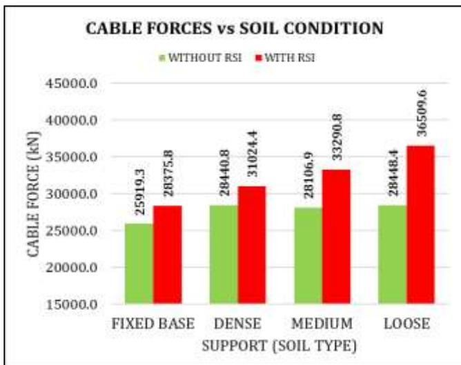
Chart -6: Cable force – 21 m pylon and HSLM A6
