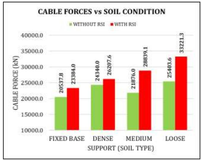
Chart -7: Cable force – 25 m pylon and HSLM A2
