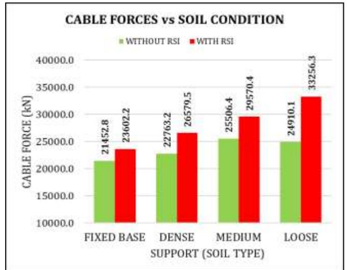
Chart -8: Cable force – 25 m pylon and HSLM A4
