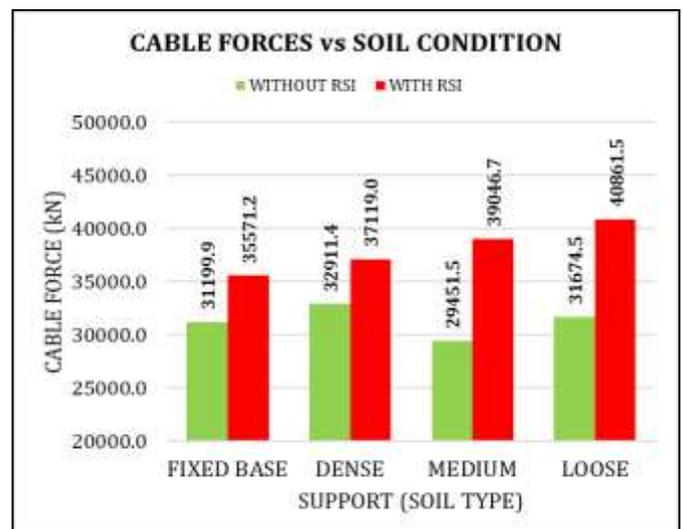
Chart -3: Cable force - 17 m pylon and HSLM A6
