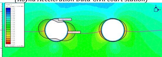
Fig.5.17 Axial force diagram
