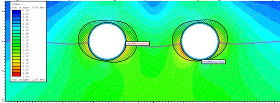
Fig.5.2 Axial force diagram (MDE Shivajinagar station)
