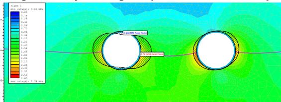
Fig.5.6 Axial force diagram (MDE Civil court station)
