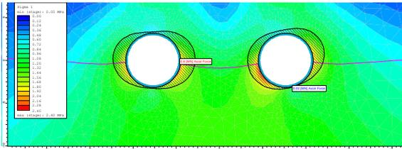
Fig.5.1 Axial force diagram (ODE Shivajinagar station)
