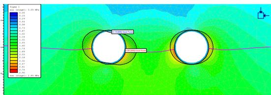
Fig.5.15 Axial force diagram
