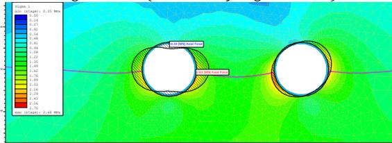
Fig.5.5 Axial force diagram (ODE Civil court station)
