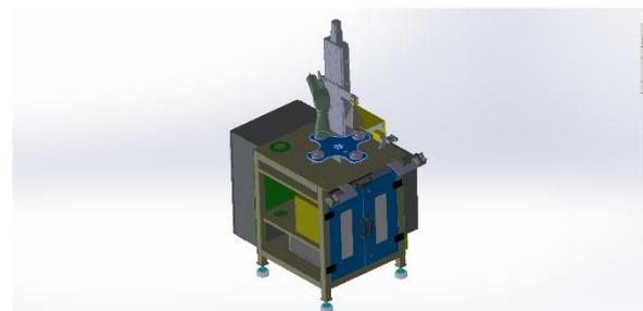
Fig-6: Rotating Fixture
