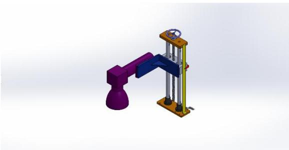
Fig-3: Laser Mount Column
