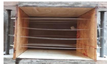
Fig 3.11: Mould with POF before pouring concrete in cube
