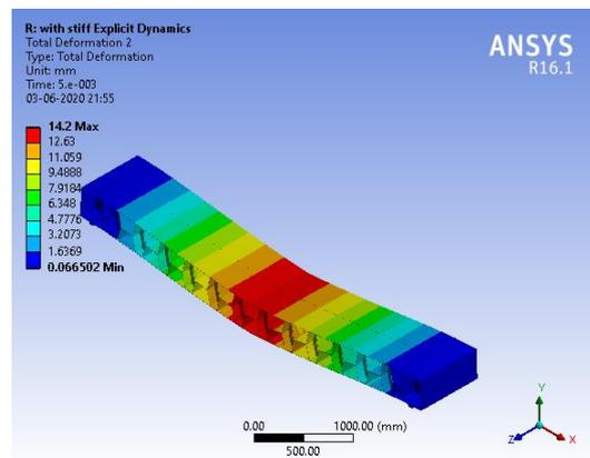
Fig -30: Total deformation of model with 1 central stiffener of depth 45mm (1S-C-d45).
