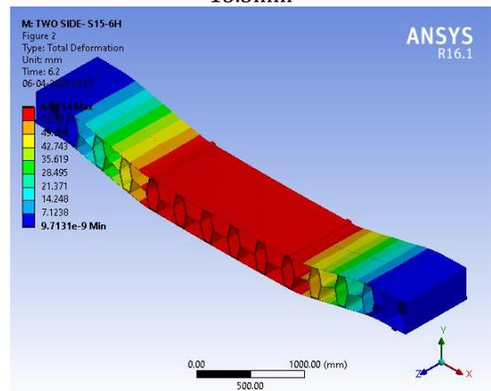
Fig -26: Total deformation of Beam model with Hexagonal folded web plate of two stiffeners one interior and one exterior
