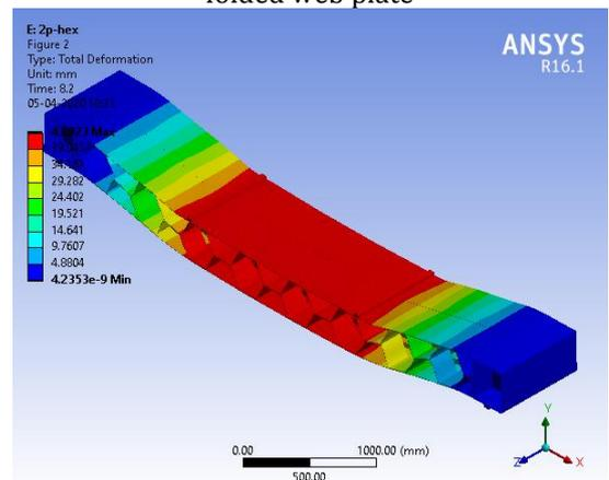
Fig -19: Total deformation of Beam model with Hexagonal folded web plate
