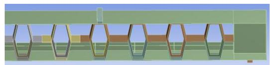
**Fig -11:** Beam model with Hexagonal folded web plate of one central stiffener of thickness 13.5mm
