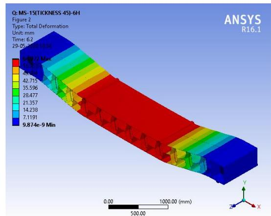
Fig -25: Total deformation of Beam model with Hexagonal folded web plate of one central stiffener of thickness 13.5mm
