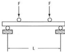
Fig -15: Four-point loading
