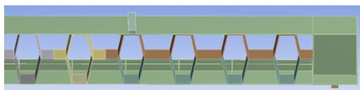
**Fig -5:** Beam model with Hexagonal folded web plate without stiffener
