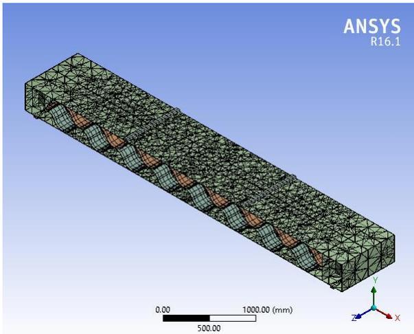
Fig -14: Meshing of 3D model in ANSYS 16.1
