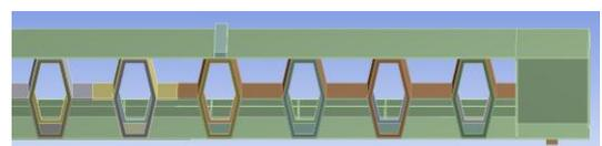
**Fig -9:** Beam model with Hexagonal folded web plate of two stiffeners one interior and one exterior
