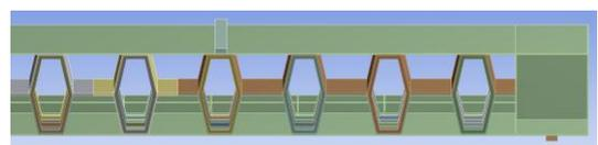
**Fig -13:** Beam model with Hexagonal folded web plate of three stiffeners, one exterior, one interior and one central stiffener
