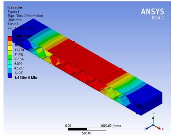
Fig -17: Total deformation of Beam model with Circular folded web plate
