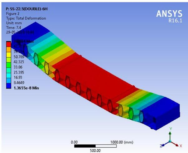
Fig -28: Total deformation of Beam model with Hexagonal folded web plate of two stiffeners one interior and one exterior of depth 22.5mm
