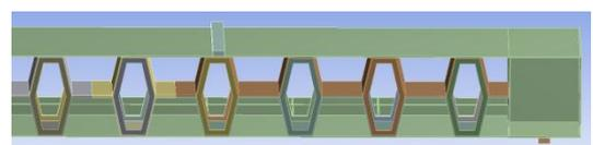
**Fig -10:** Beam model with Hexagonal folded web plate of two stiffeners one interior and one exterior of depth 22.5mm
