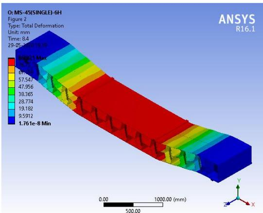
Fig -27: Total deformation of Beam model with Hexagonal folded web plate of one central stiffener of depth 45mm
