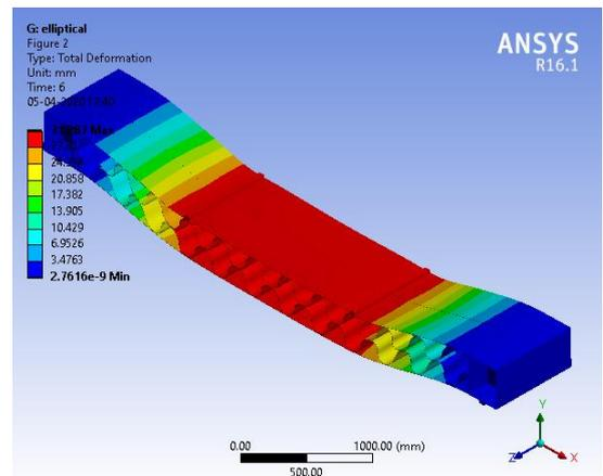
Fig -18: Total deformation of Beam model with Elliptical folded web plate
