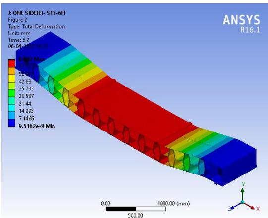
Fig -21: Total deformation of Beam model with Hexagonal folded web plate of one exterior stiffener
