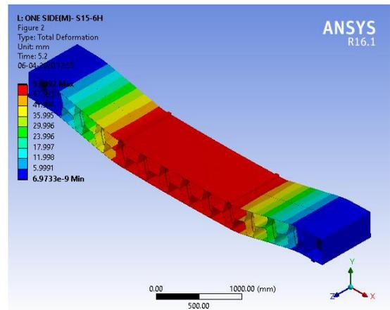
Fig -24: Total deformation of Beam model with Hexagonal folded web plate of one central stiffener
