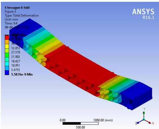
Fig -20: Total deformation of Beam model with Hexagonal folded web plate without stiffener
