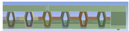
**Fig -12:** Beam model with Hexagonal folded web plate of one central stiffener of depth 45mm
