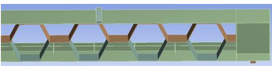
**Fig -4:** Beam model with Hexagonal folded web plate
