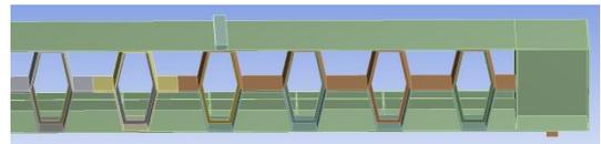
**Fig -7:** Beam model with Hexagonal folded web plate of one central stiffener
