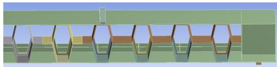
**Fig -8:** Beam model with Hexagonal folded web plate of one interior stiffener
