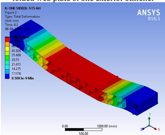
Fig -22: Total deformation of Beam model with Hexagonal folded web plate of one interior stiffener
