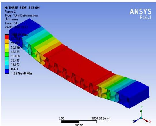
Fig -29: Total deformation of Beam model with Hexagonal folded web plate of three stiffeners, one exterior, one interior and one central stiffener
