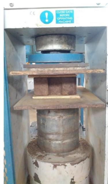
**Figure -3:** Interlocking block specimen placed on the compressive test machine
