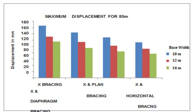
Chart 4: Comparison of Maximum Displacement for Tower Height: 80m
