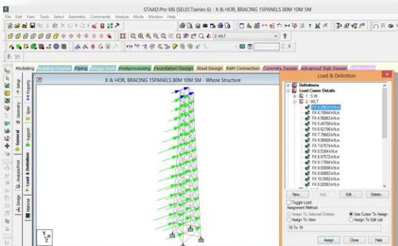
Fig 6: Typical view of wind load acting on a structure
