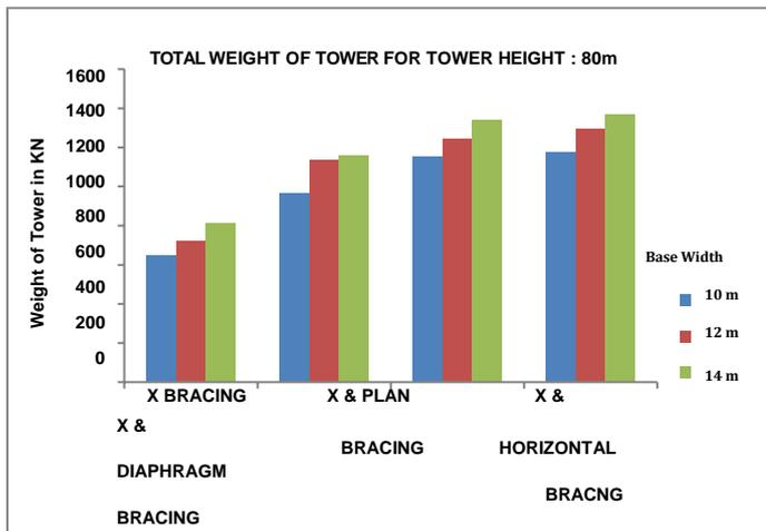
Chart 5: Comparison of Total Weight of Tower for Tower Height: 80m
