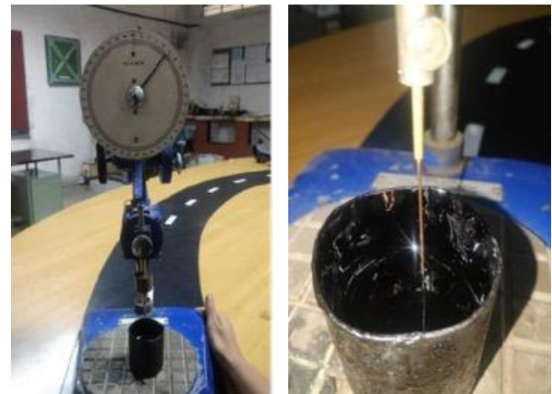
Fig -9 & 10: Penetrometer & Sample Testing
