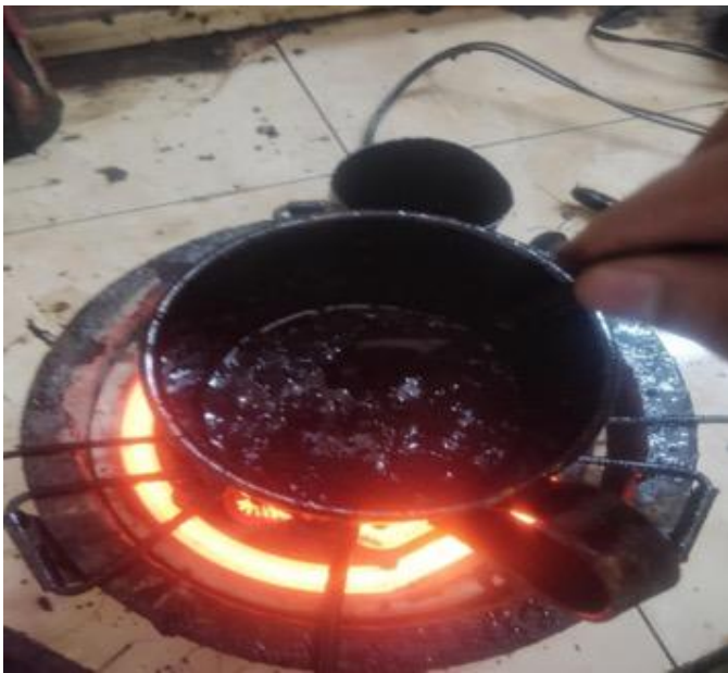
Fig -5: Heating Bitumen.
