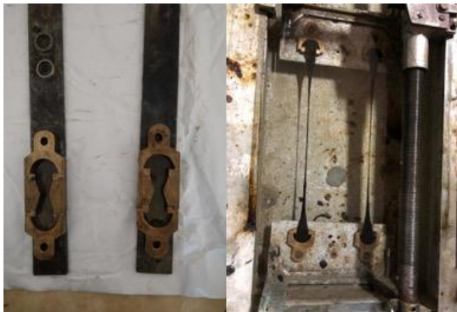
Fig -15: Ductility Test Specimen and Sample Testing Mold
