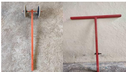
Fig.7: Front wheel assembly and Pull handle
