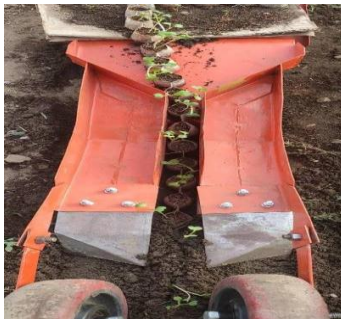
Fig.3: Working of paper pot transplanting machine
