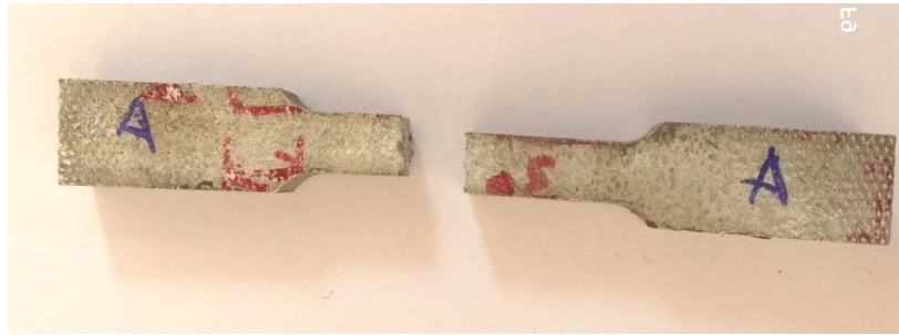
Figure 2 Failed Tensile Testing Specimen
