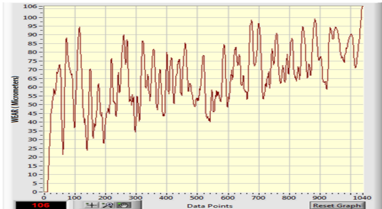
Figure 3 Wear of AMMC Specimen at 6% Reinforcement
