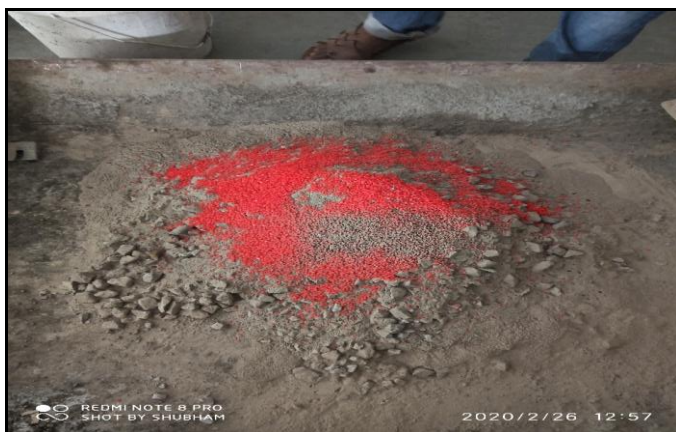
Figure 2: Addition of plastic granules
