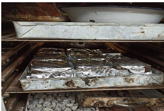
Figure 3: Oven curing of samples
