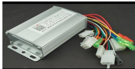
Fig -4: Motor controller
