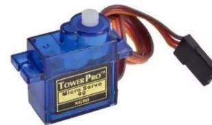
This SG90 360 degree Continuous Rotation Servo Motor is special among all the available servo motors because its operation is very different from that of a standard servo. As instead of going to a specified angle, this servo will be static at a 1.5ms pulse, a longer pulse gives forward rotation and a shorter pulse give backward rotation.
